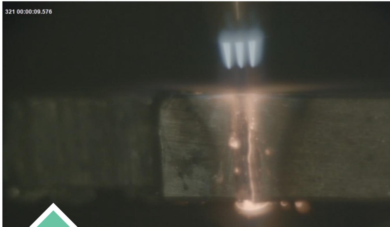
On the top, an image of oxyacetylene cutting taken by a Xiris weld inspection camera. On the bottom, an image of oxyacetylene cutting taken by a standard camera. With the Xiris camera, users are able to see great detail throughout the cutting flame, whereas the standard camera simply saturates and blooms.
