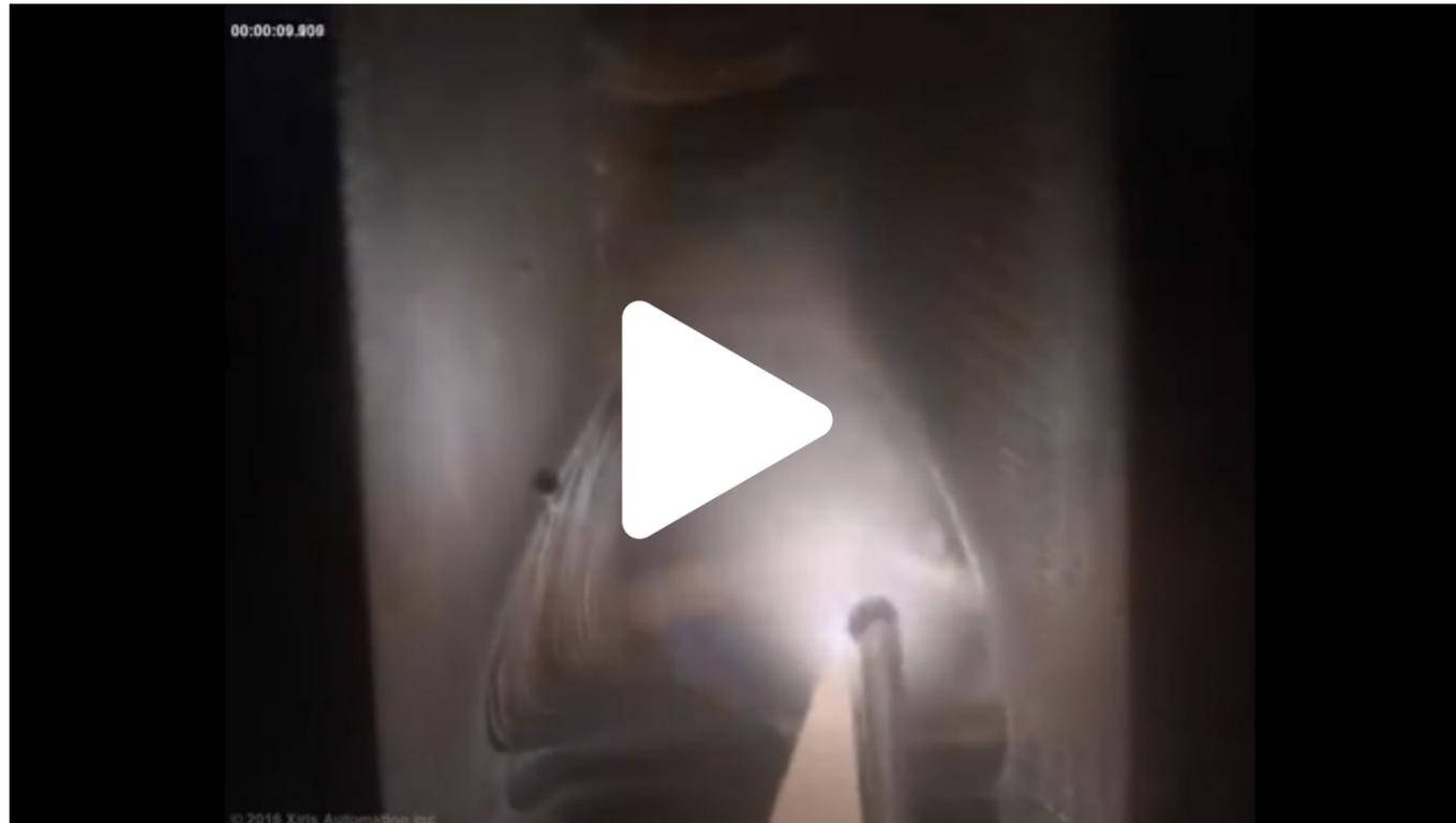
In this video, Xiris weld inspection cameras capture manual TIG welding on a rotary pipe in the vertical up position.
