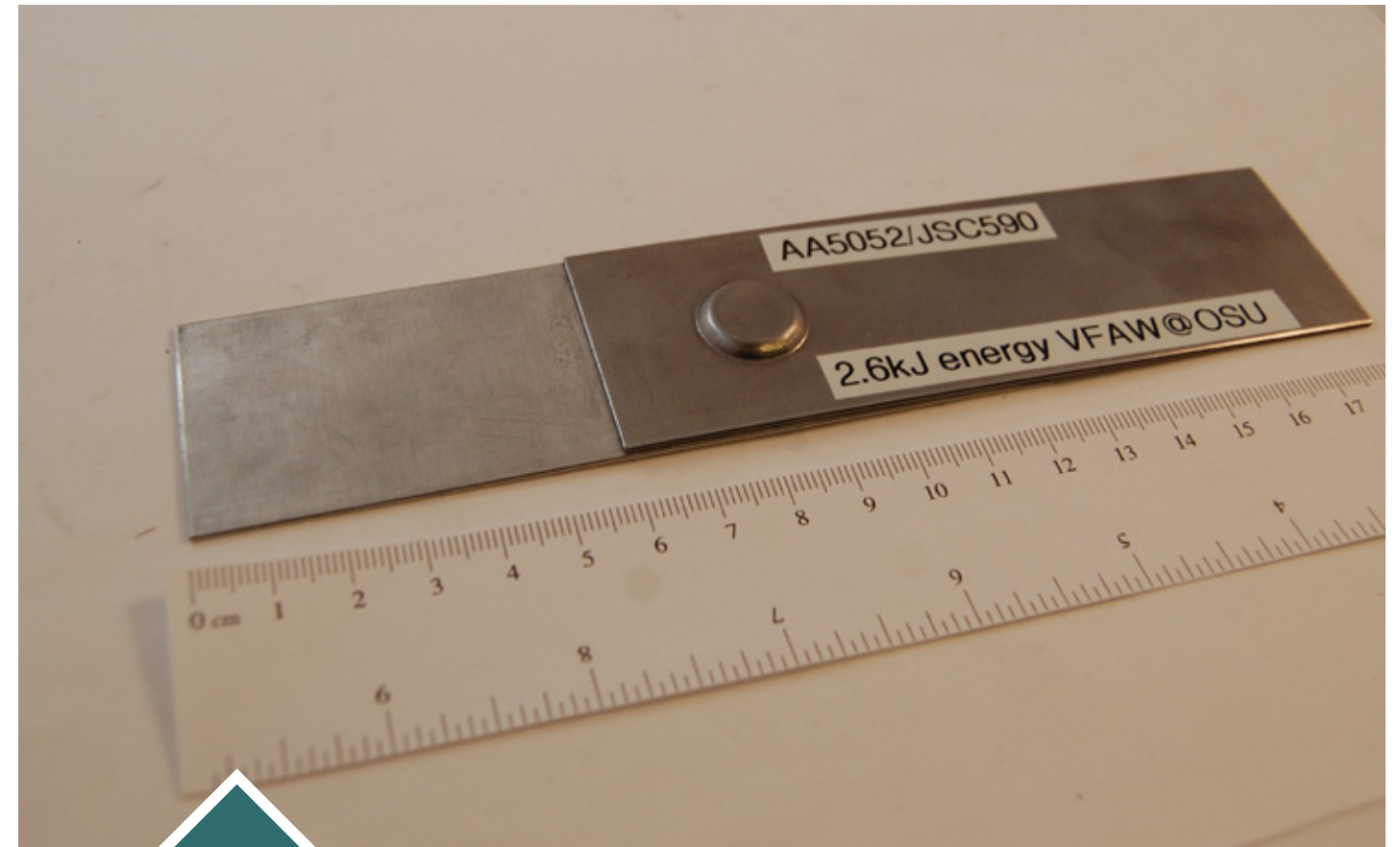
Impact spot welding achieves what other types of welding or adhesives cannot: joining dissimilar materials at a lower cost.
