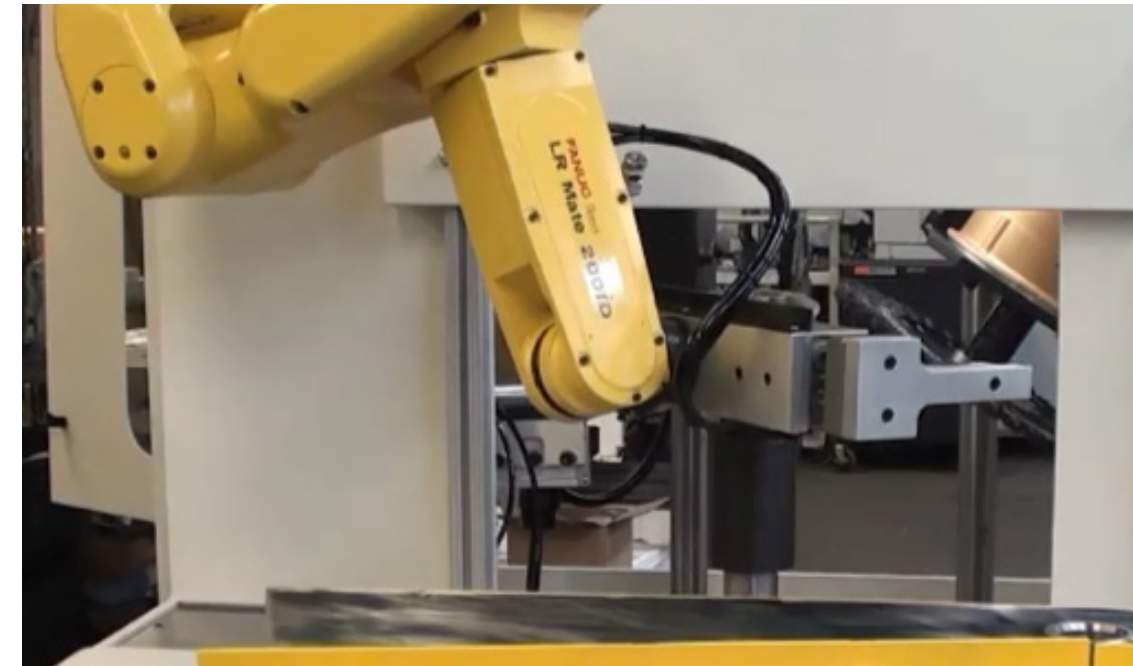
A deburring machine with robotic loading and unloading.
