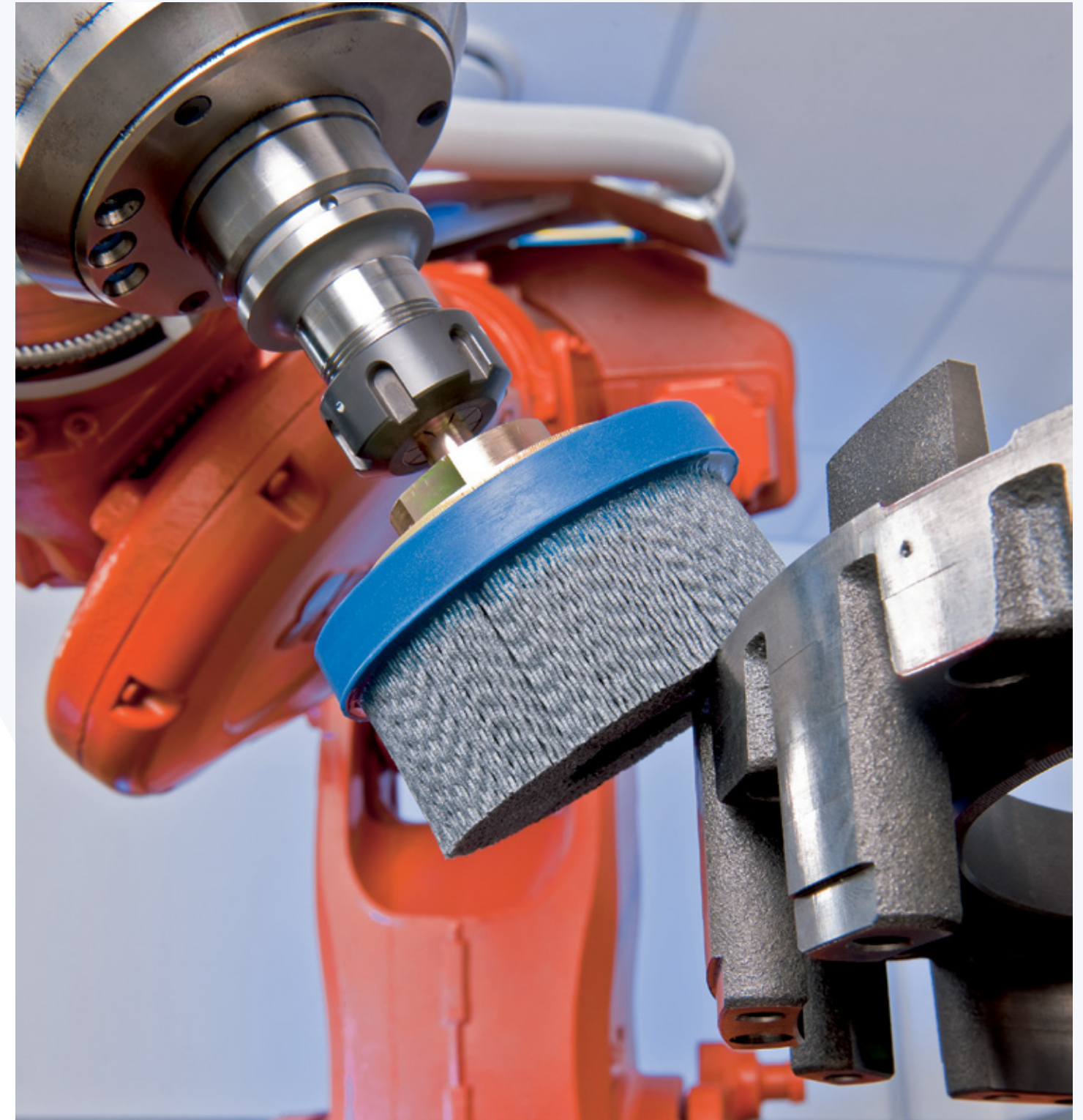
A robot performing a deburring process using an M-Brad abrasive filament brush.
