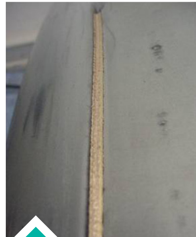
Thanks to the even outflow of the copper wire, the seam created by laser brazing can hardly be seen later.
