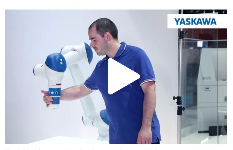
Watch this video to see how the robotic arm shuts down if the operator comes in contact with the HC10 while it is in motion.
