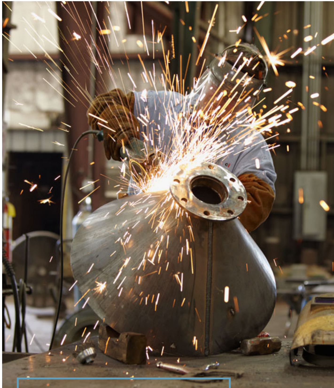
A custom cone segment with flanges during the cutting phase.
