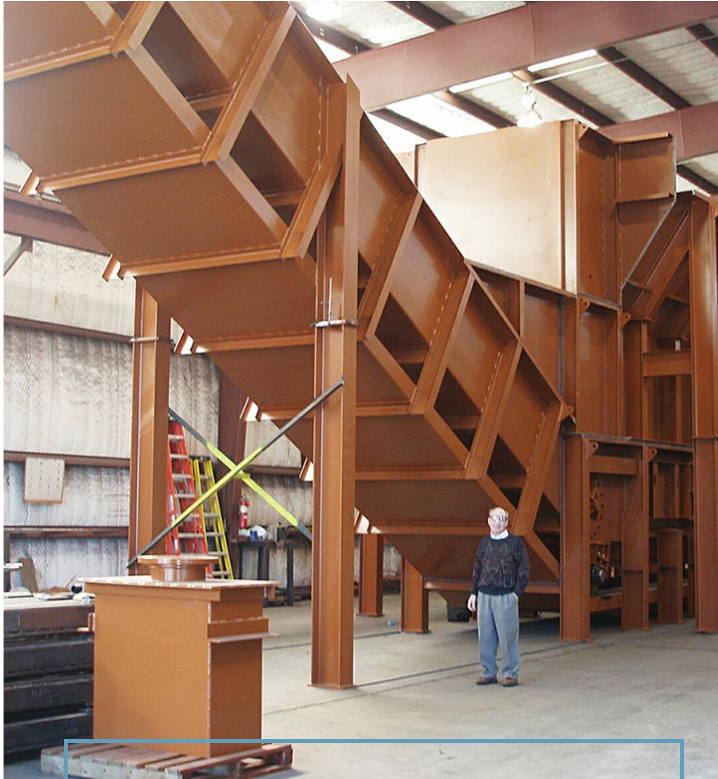
A 127-ft. submerged scraper conveyor designed and fabricated to mate with a transition chute for removing bottom ash at a utility power plant.
