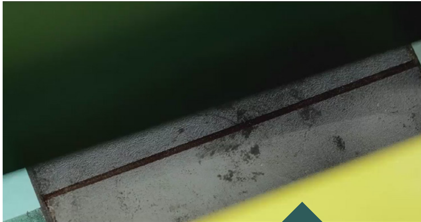
The urethane hold-down allows the operator to look over the hold-down bar and find the cut mark on the workpiece.
