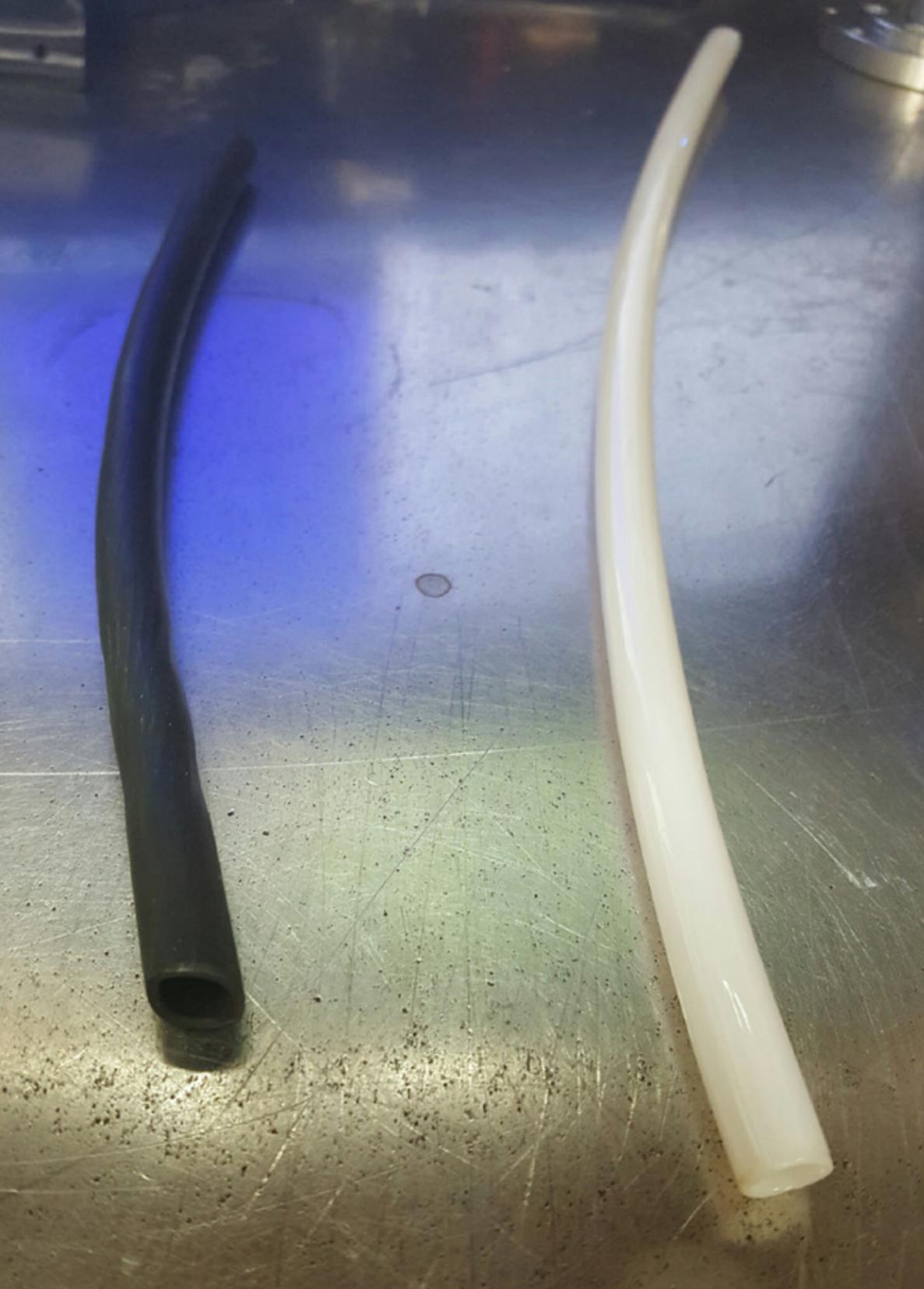
For the MIG cable inner tube, Hytrel makes the inner tube kink resistant, although a black synthetic rubber inner tube is still a good option.
