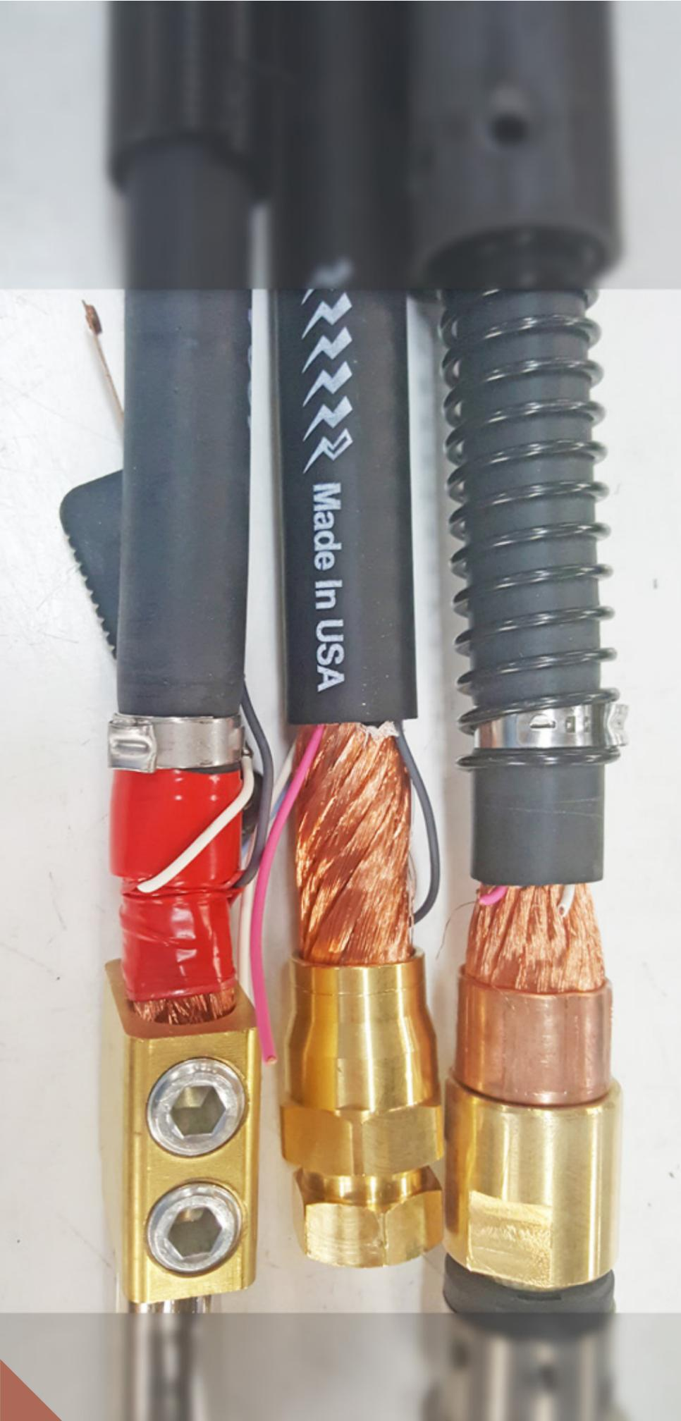
Manufacturers use crimp connections (right), set screws (left) or cone and nut compression-type fittings (middle) for cable guns.
