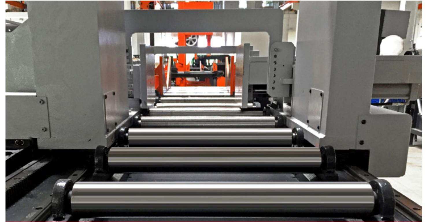
↑ The feeder component of the AV-2026NC, along with the Mechalogix software Cosen has developed, allows operators to program in (i.e. index) nearly 1,000 in. of material for processing.
