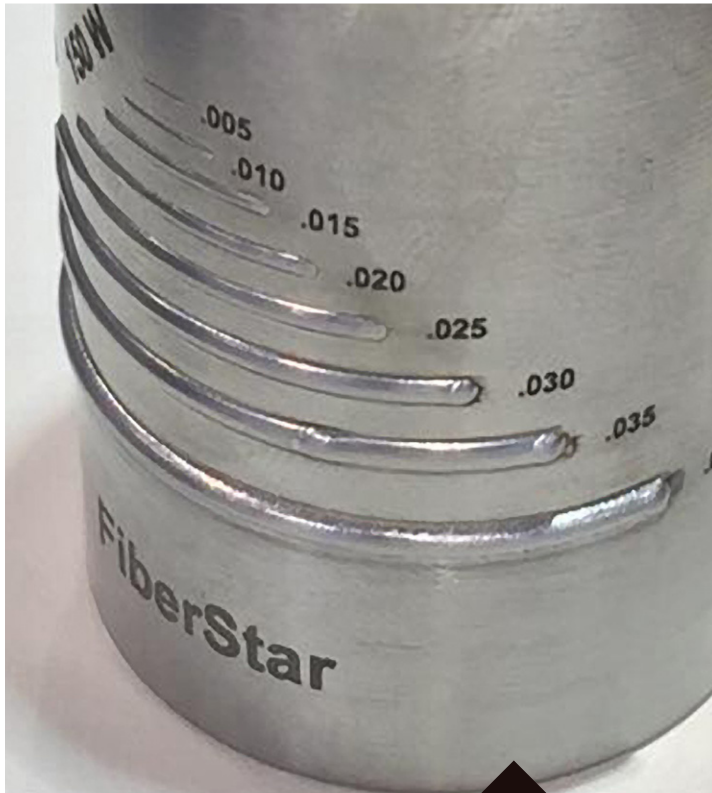
With wires from 0.005 in. to 0.045 in., LaserStar's FiberStar line offers flexibility in welding small parts.
